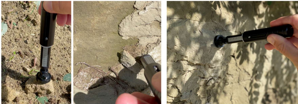
Pocket penetrometer assessment of the cohesion for various zones of the slopes
